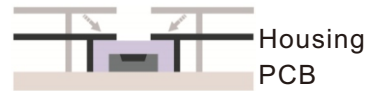
Figure 13: Small measurement dead zone helps the sensor to quickly and comprehensively detect environmental changes.
