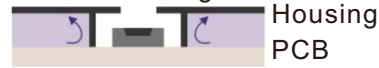
Figure 12: The sensor is isolated from the air inside the housing, which minimizes the impact of the air inside the housing on the sensor.
