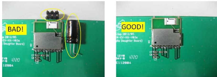
Figure 2-26: First Example of bad and good GNSS module placements
