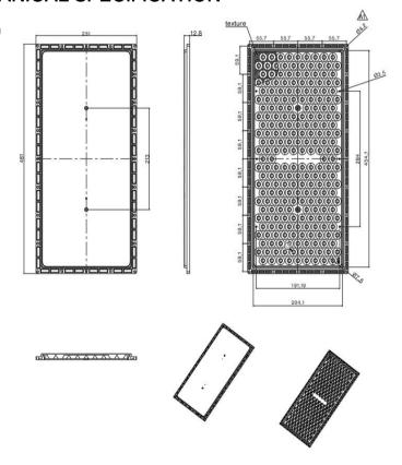
Dimensions with unmarked tolerances refer to GBT14486 tolerance table.
