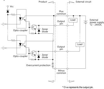
The signal output section is an opto-coupler isolated, open-collector output (current sink type). Driving the output section requires an external power supply.
