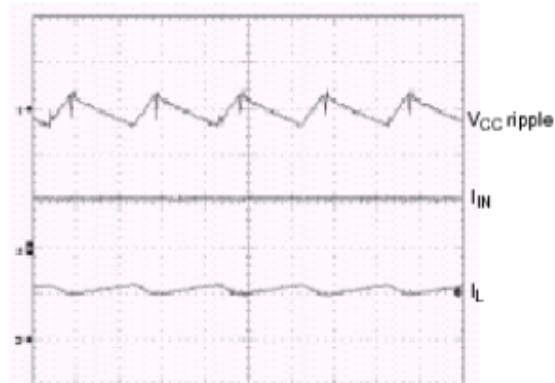
Figure 25. Boost Input Voltage and Current Ripple Waveforms
