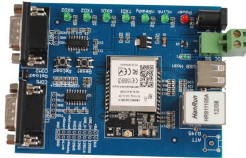
Figure 6. HF-A11-SMT Evaluation Kit
